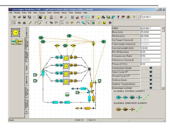
LES software can be used to create the initial engine model
