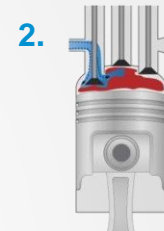
2. Top Dead Centre Air injected - comes into contact with the HEF causes rapid temperature rise.
