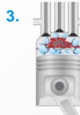
3. Power Stroke The air expands pushing the piston down. Direct contact heat transfer continues allowing near isothermal expansion.
