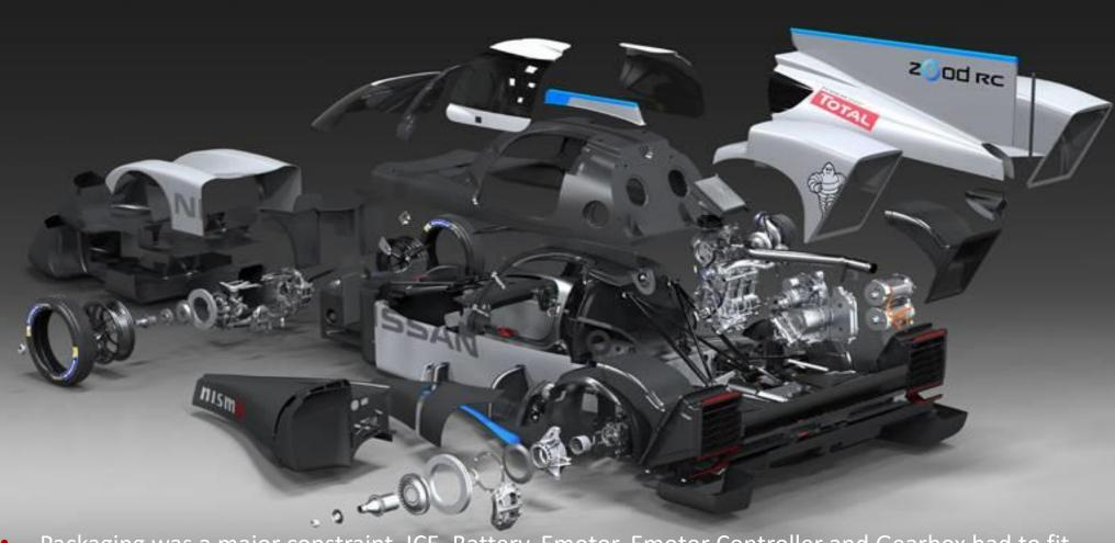
• Packaging was a major constraint, ICE, Battery, Emotor, Emotor Controller and Gearbox had to fit into limited space for the low drag configuration.
