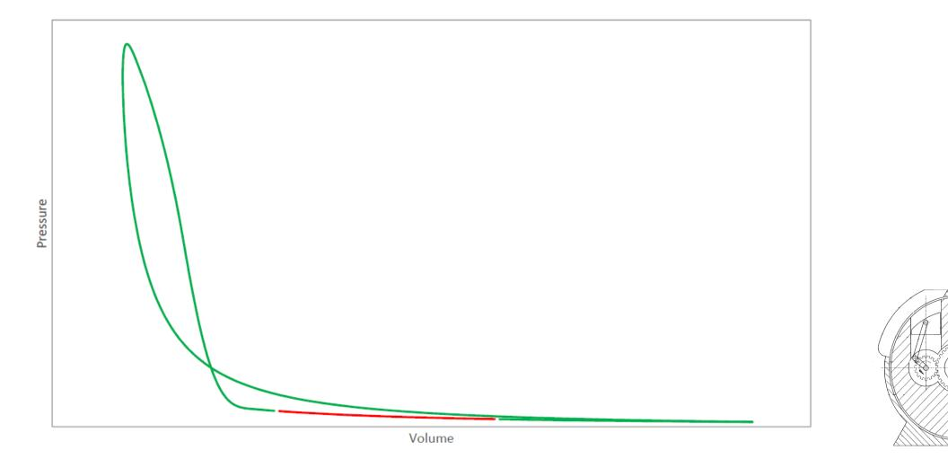
1: Positive Work at beginning of the Compression Stroke
