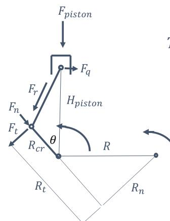
$Torque = F_t.R_t + F_n.R_n + F_q.H_{piston}$  $= F_t.(R_{cr} + R.Sin\theta) + F_n.R_n + F_q.H_{piston}$
