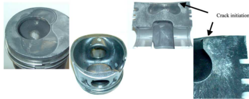
Fig. 5. Diesel engine piston with a crack from one side of the pin hole to the other pin hole going through the head of the piston.
