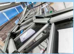
Such packages are no problem for EuroSort's split-tray sorters, which are ideal for mixed mail. The solution will be on show throughout POST-EXPO 2018, alongside the company's robot arm, which will show the technical possibilities for picking from boxes or totes and inducting in the sorter machine automatically.
